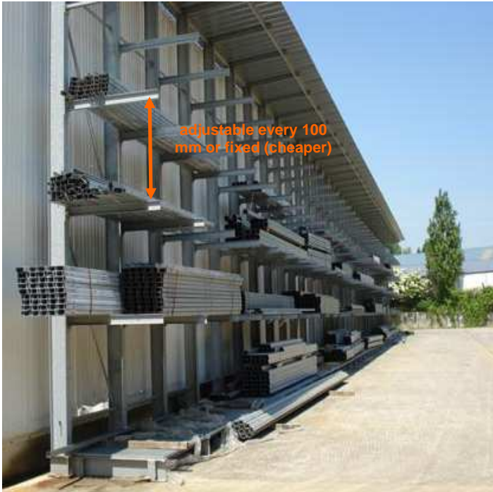
Galvanized RediCant® with roof for exterior storage.
